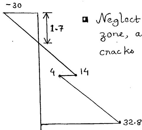
■ Neglect tension zone, as tension cracks develop.
