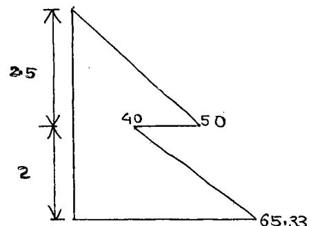
$$P_a = \frac{1}{2} \times 50 \times 2.5 + 2 \left( \frac{40+65.33}{2} \right) = \underline{\underline{167.8 \text{ kN/m}}}$$
