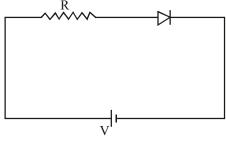
(a) In forward biasing the voltage across R is V
