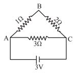
Here, two reisistance of  $1\Omega$  and  $2\Omega$  are in series, which form  $3\Omega$  which is in parallel with  $3\Omega$  resistance.
