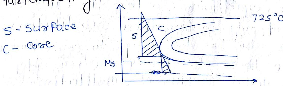
Austenite sample is quenched into a hot bath maintained at a temp. below the nose and above  $M_s$ . Sample is kept at this temp. for certain period of time so that temp. b/w surface and core becomes uniform. sample is then taken out from hot bath and quenched into a cold bath maintained at room temp. Martempering is decrease temp.
