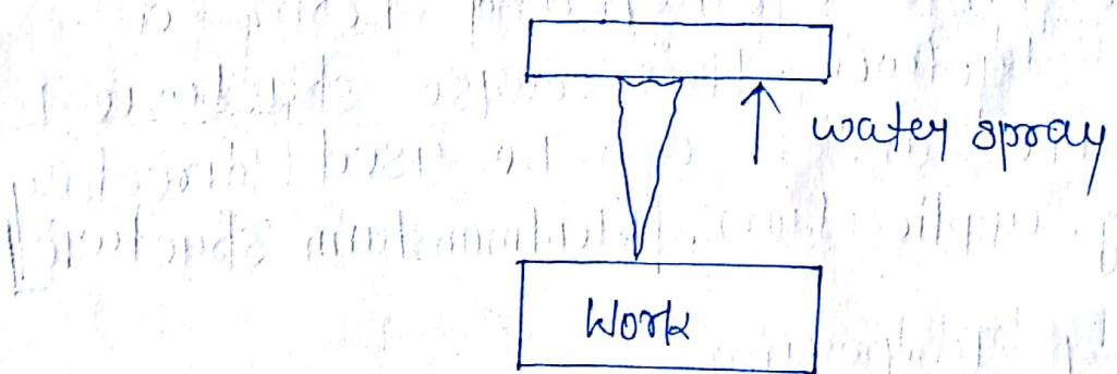
cam shaft are case hardened by frame hardening. By this technique, medium 'c' steel material are heated by oxidizing flame and then immediately quenched with water. This produce a thin layer of M over specimen.
