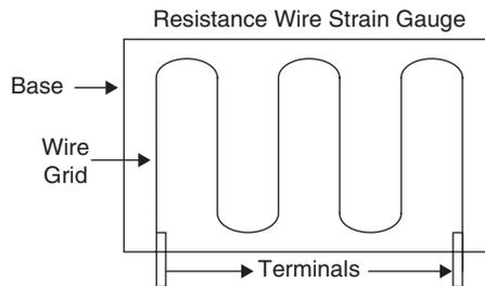
Consider a strain gauge made of circuit wire.
