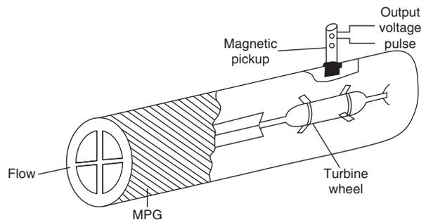
It is used in the measurement of liquid gases and gases of very low flow rate. It consists of a multi bladed rotor called the turbine wheel which is mounted 90° to the axis of flowing liquid.
