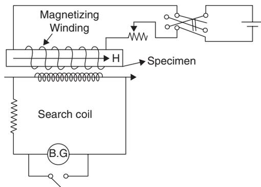
The value of flux density  $B_0$  in search coil is measured in a similar manner described above for determination of  $B$  in the specimen.
