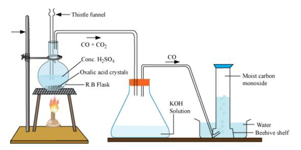
Pour concentrated sulphuric acid from thistle funnel so that the lower end of thistle funnel is completely immersed in acid. Heat the mixture.
