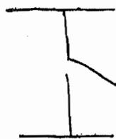
$$A \rightarrow \overline{A} \quad Y = \overline{A}$$
