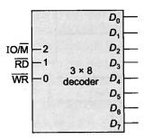
If this to be used with 8085 to generate read and write control signals then valid outputs are
