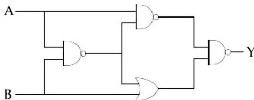
**Q.No. 29** The output of the given logic circuit is :
