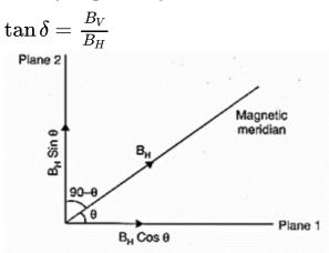
Let  $\delta_1$  be the (apparent) dip in a plane which makes angle  $\theta$  with the magnetic meridian. In this plane, the vertical component will be  $B_V$  only but the effective
