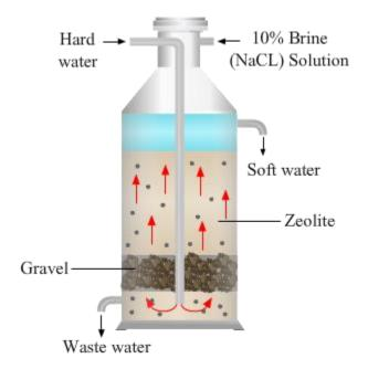
(iii) In the column given in the figure, sand, gravel and permutit are placed in alternate layers through which hard water flows down. As water passes, Ca<sup>2+</sup> and Mg<sup>2+</sup> ions are exchanged with Na<sup>+</sup> ions of the permutit. This forms calcium and magnesium permutit leaving behind only pure water.
