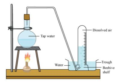
Heat the water in the round bottomed flask. After some time, some tiny bubbles of gas coming out of the water are observed. If the heating is continued, then water starts boiling and the gas bubbles start coming out of the beehive shelf. Lower the flame to keep the water just near the boiling point. Then invert a graduated tube completely filled with tap water over the beehive shelf. The boiled off air starts collecting in the tube by replacing water.
