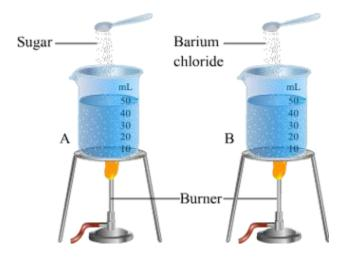
**Procedure:** Take two beakers and label them A and B. Fill each with 50 mL of water. Dissolve sugar in beaker A and barium chloride in beaker B. Keep dissolving the solutes in the respective beakers till the solutions become saturated and no more solute can be further dissolved. After this, heat the solutions and dissolve one more spatula of the solutes in the respective beakers. Slowly cool down the solutions after the solutes added further get completely dissolved.
