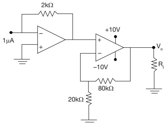
**10.** Find the voltage gain of below circuit?
