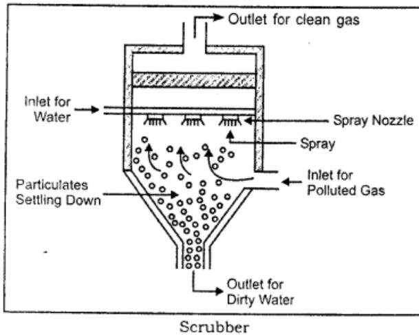
during emissions. In this process, water is introduced into a spray tower by means of a spray nozzle which allow downward flow of water. As the polluted gas flows upwards, the particulates present in the gas collide with the water droplets being sprayed from the spray nozzles. Under the influence of gravitational force, the liquid droplets containing the particulates settle at the bottom.
