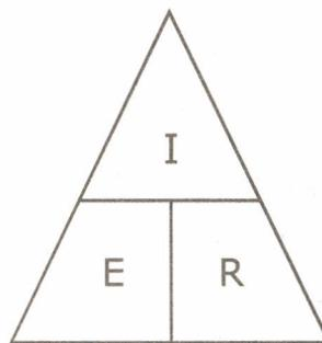
Fig: 5.5 Triangular of Voltage, Current, Resistance
