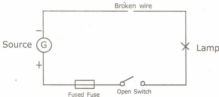
Fig:5.3 Open Circuit
