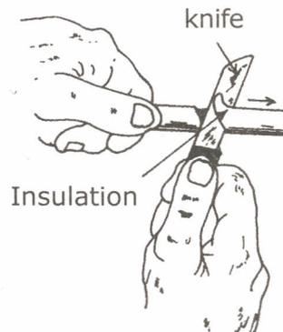
Fig: 6.2 Striping Insulation
