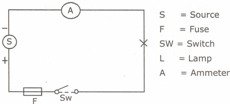
Fig: 3 Connection of ammeter.
