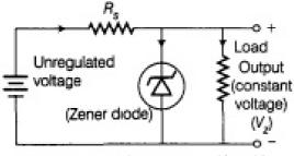
Excess current bypass when  $V_{ext} \ge V_z$
