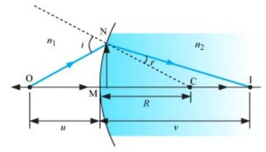
The above figure shows the geometry of formation of image / of an object O and the principal axis of a spherical surface with centre of curvature C and radius of curvature R.
