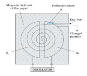
Working Principle: The cyclotron uses crossed electric and magnetic fields which increases the kinetic energy of a charged particle without changing its frequency of revolution.
