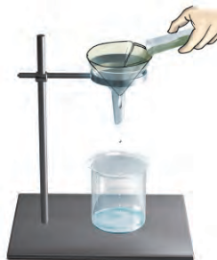
Fig. 5.10 Filtration using a filter paper
