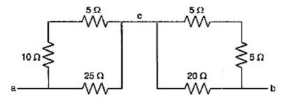
The left block is equivalent to 15 ohm and 25 ohm in parallel
