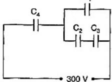
So, voltage across  $C_4$  is 200 V. The voltage across the combination of  $C_1$ ,  $C_2$  and  $C_3$  is 100 V. Since  $C_1$  and  $C_{23}$  are in parallel, therefore, the voltage across  $C_1$  as well as across the series combination of  $C_2$  and  $C_3$  is 100 V. Again,  $C_2$  and  $C_3$  are equal therefore, 100 V would be shared equally between  $C_2$  and  $C_3$ .
