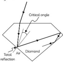
The total internal reflection of the light is used in polishing diamonds to create a sparking brilliance. By polishing the diamond with specific cuts, it is adjusted the most of the light rays approaching the surface are incident with an angle of incidence more than critical angle. Hence, they suffer multiple reflections and ultimately come out of diamond from the top. This gives the diamond a sparking brilliance.
