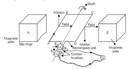
In the figure, coil ABCD is placed in the magnetic field. The coil ABCD is horizontal initially. It is made to rotate in the clockwise sense and the arm AB moves up while CD moves down. According to Fleming's right hand rule, the direction of the induced current will be along ABCD. When the coil completes half rotation, the arm CD moves up and AB moves down. Now the direction of the induced current is opposite along DCBA.
