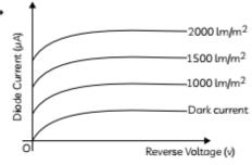
The voltage-ampere characteristic curve for three different values of Ge photodiode. Only dark current passes through origin. Current increases with increase in illumination for a given reverse voltage.
