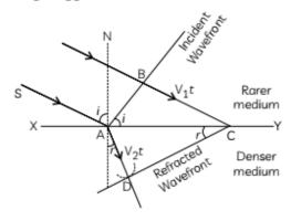
Let a wavefront AB incident on a plane surface XY, separating two media 1 and 2. Let  $V_1$  and  $V_2$  be the velocities of light in two media such that  $v_1 > v_2$ .
