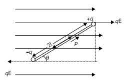
When an electric dipole is kept in an external uniform electric field, a couple acts on it, which tries to align the dipole in the direction of the field. This is called the restoring couple.
