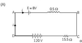
When a battery is charged by using an external D.C. supply current will flow from positive terminal of battery to the negative (i.e. in the reverse direction).
