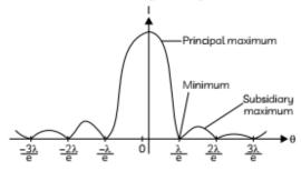
In diffraction pattern a central bright band having on both sides narrower alternately dark and bright bands of decreasing intensity will obtain. If the intensity of the central maxima is  $l_0$  then the intensity of the first and second secondary maxima are found to be  $\frac{l_0}{22}$  and  $\frac{l_0}{61}$ .
