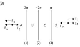
Given, thin long sheets have surface charge density  $+2\sigma$ ,  $-2\sigma$  and  $+\sigma$  respectively. We need to calculate electric field intensity at point A and point D.
