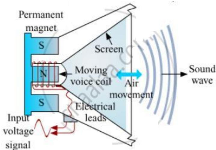
Now, when variable current flows through the coil, magnetic field is produced around it due to electromagnetism and it behaves like an electromagnet. Because of this, the coil is repelled and attracted by the permanent magnet alternately. The screen attached to the coil moves back and forth due to the attraction and repulsion of the coil and hence, produces sound.
