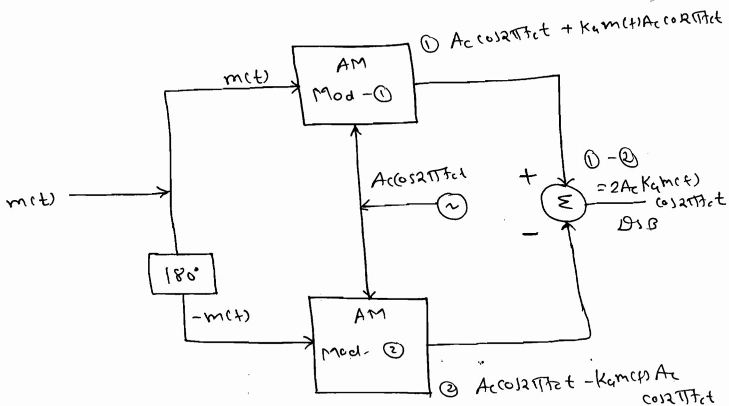
⇒ "Balanced modulation can be used as "multiplier!"
