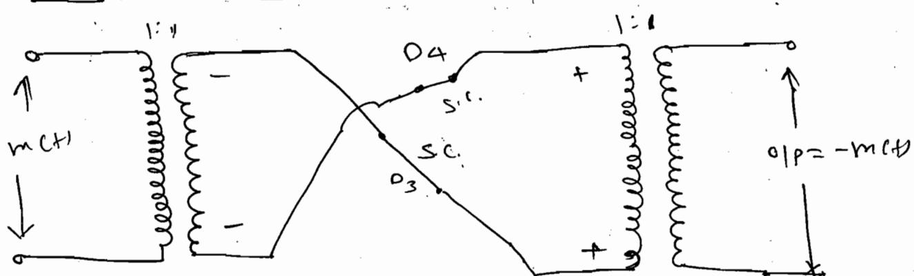
⇒ In DSB when carrier signal changes its polarity (or) crosses 'zero' line then there will be  $180^\circ$  phase shift in DSB signal.
