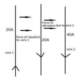
The magnetic field caused by a long wire is given by  $B = \frac{\mu_0 i}{2\pi d}$  where i is the current in the wire, d is the distance at which B is to be calculated,  $\mu_0$  is the magnetic permeability of free space. Let the distance between the two wires be 2d.
