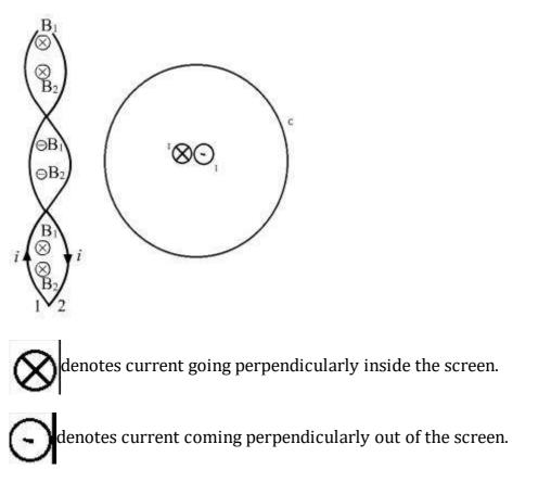
If this both currents are equal in magnitude then the total current enclosed by the Amperian Loop C will be zero.
