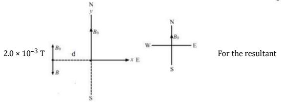
magnetic field to be zero, we need to have a field in opposite direction to that of the existing field. Hence, magnetic field B due to wire in the direction from north to south as shown in the diagram. **Formula used:** By Ampere's Law for a current carrying wire is  $B = \frac{\mu_0 i}{2\pi d}$  Where,
