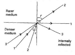
makes refracting angle 90° and light cannot escape the denser medium. So angle is the critical angle. From Snell's law,  $i = i_c$ , r = 90°
