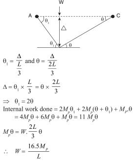
The collapse load will be minimum of above two values So; collapse load =  $\frac{15M_p}{L}$ . Choice (C)
