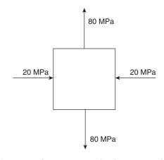
For the state of stress at a point in a stressed body, shown in figure radius of the Mohr's circle is (A) 80 MPa (B) 60 MPa
