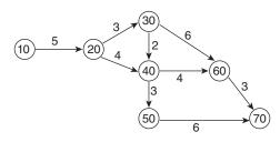
For the network shown in figure, find the critical path?
