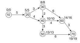
**Critical path**: 10 - 20 - 30 - 40 - 50 - 70 (or) Critical path is the path along which duration is maximum. From options, the path 10 - 20 - 30 - 40 - 50 - 70 has maximum duration. Choice (B)
