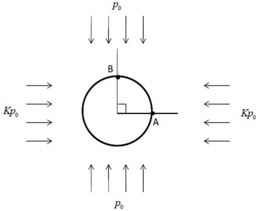
If the ratio of the tangential stress measured at the boundary points A and B is 3:1, the value of  $K$  is
