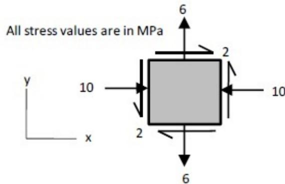
The magnitude of the maximum shear stress in MPa and its direction with the  $x$ -axis in degrees at the same point respectively are
