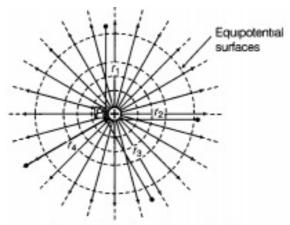
Equipotential surfaces for a point charge
