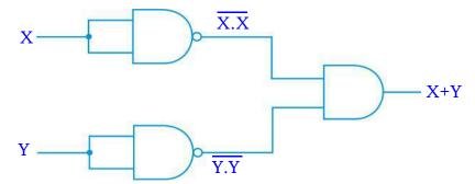
X + Y = (X NAND X) NAND (Y NAND Y) Proof : X NAND X =  $\overline{X}$ .  $\overline{X}$  =  $\overline{X}$  +  $\overline{X}$
