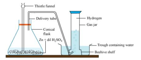
Pour 2 cc of copper sulphate solution through the thistle funnel, and then dilute sulphuric acid, so that the lower end of the thistle funnel is completely immersed. Then, a reaction takes place between zinc and sulphuric acid, with the evolution of hydrogen gas. Here, the copper sulphate solution acts as a catalyst.
