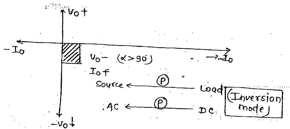
\* Inversion mode can be used for regenerative braking of a dc m/c.
