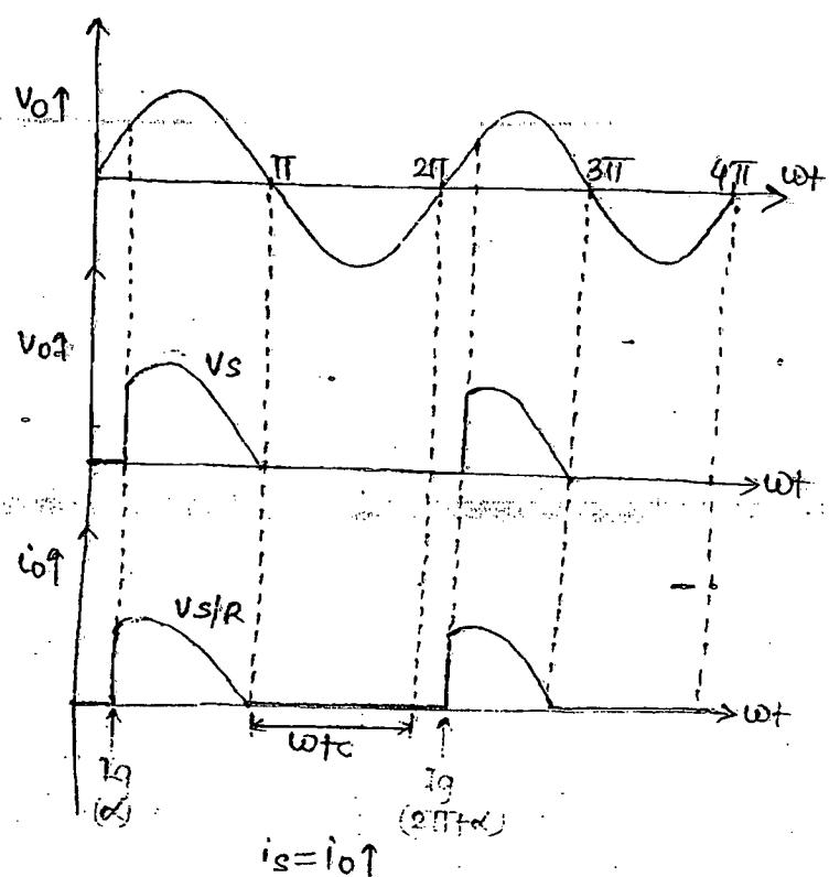
Drawback → The source current contains dc components & saturates the supply T/F core.
