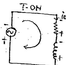
\* Here the inductance energy makes the thy. to conduct even in the -ve cycle until it releases its complete energy at  $\omega t = \beta$
