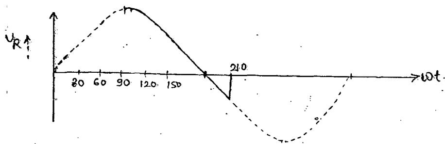
$$\alpha = 60^\circ, wt = 90^\circ, \text{ end } 90 + 120 = 210^\circ$$
