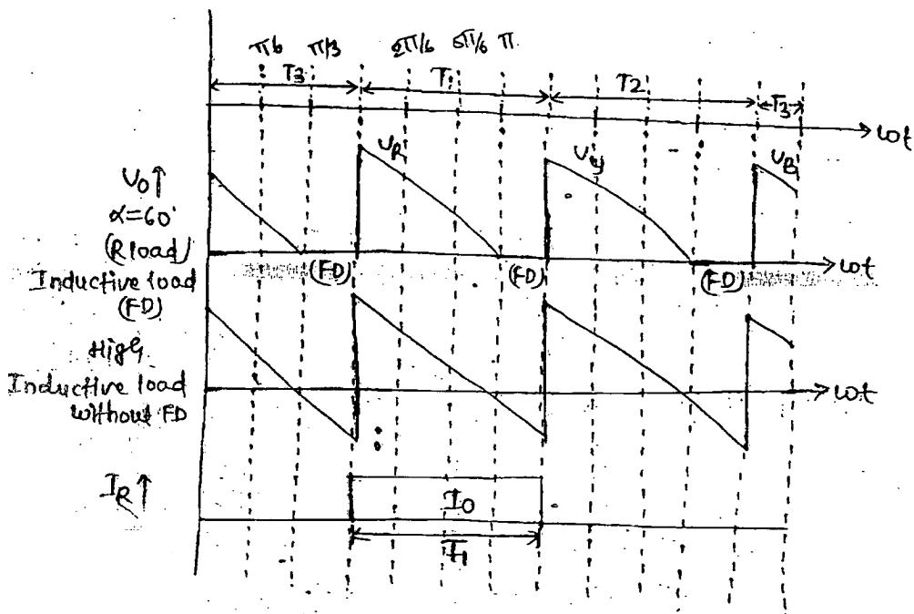
(2.)  $\alpha > 30^\circ$ : discontinuous conduction for R load :-
