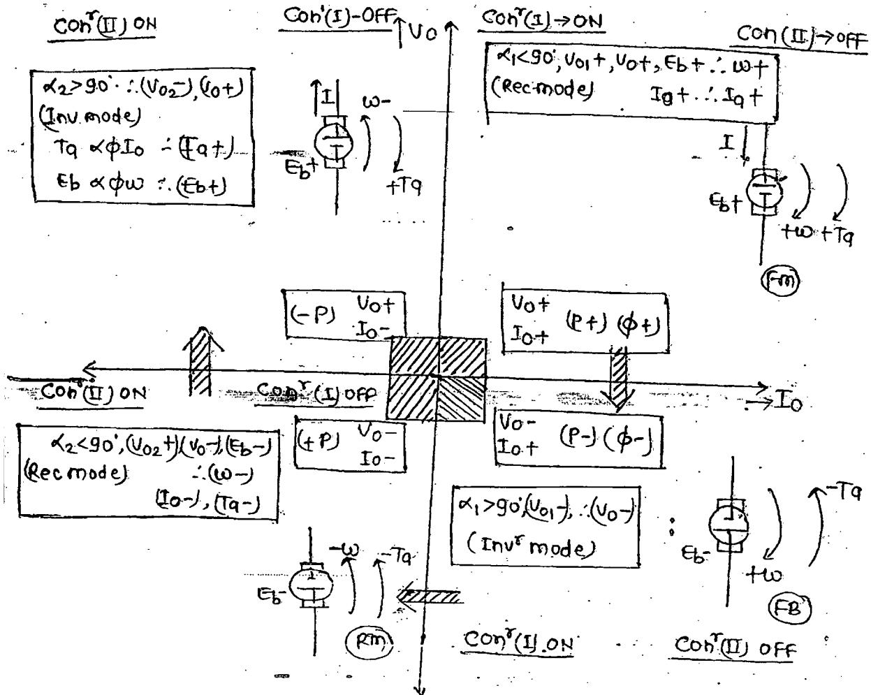
\* Disadvantage:- It gives slow speed response & the reversal of arm current is not smooth during switching operation of the cont.
