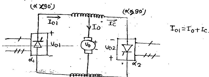
Advantage → It gives high speed response & reversal of arm. current is smooth during switching operation at con.
