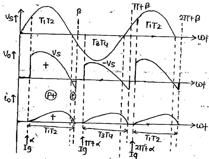
$$V_{0\alpha} = \frac{V_m}{\sqrt{2\pi}} \left[ (\beta - \alpha) + \frac{1}{2} (\sin 2\alpha - \sin 2\beta) \right]^{1/2}$$
