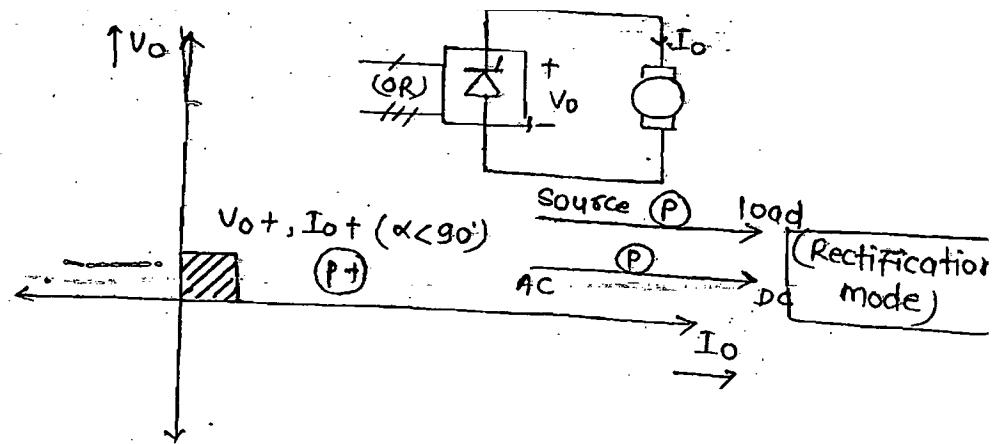
\* Rectification mode can be used for motoring mode of a dc m/c & charging battery,
