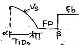
$$U_o = \frac{1}{\pi} \left[ \int_{\alpha}^{\pi} V_m \sin \omega t d(\omega t) + \int_{\pi}^{\beta} \omega d(\omega t) + \int_{\pi}^{\pi+\alpha} E_b d(\omega t) \right]$$
