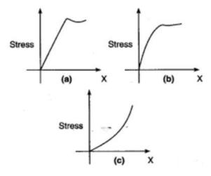
**Ans.** (b) is more brittle. A material is said to be brittle if there is small stress-strain variation beyond elastic point and fracture point of brittle material lies close to elastic point.
