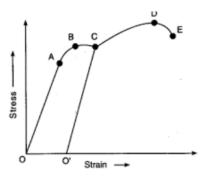
(a) Upto which point of curve, is Hooke's law obeyed? This point is also called ' Proportion limit'.
