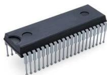
An integrated circuit (ICs), sometimes called a chip or microchip, is semiconductor wafer on which thousands or millions of tiny resistors, capacitors and transistors are fabricated. An IC can function as an amplifier, oscillator, timer, counter, computer
