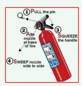
**Step 4: Sweep** the nozzle from side to side, aiming at the base of the fire. Continue until the fire is extinguished.
