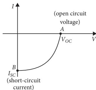
(i)  $V-I$  curve is drawn in the fourth quadrant, because a solar cell does not draw current but supply current to the load.
