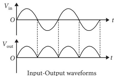
Since in both the half cycles of input a.c., electric current through load  $R_L$  flows in the same direction, so d.c. is obtained across  $R_L$ . Although direction of electric current through  $R_L$  remains same, but its magnitude changes with time, so it is called pulsating d.c.
