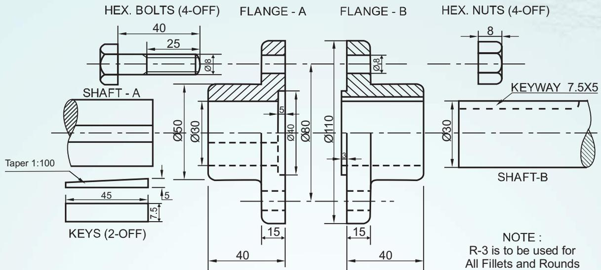
DETAILS OF AN UNPROTECTED FLANGE COUPLING
