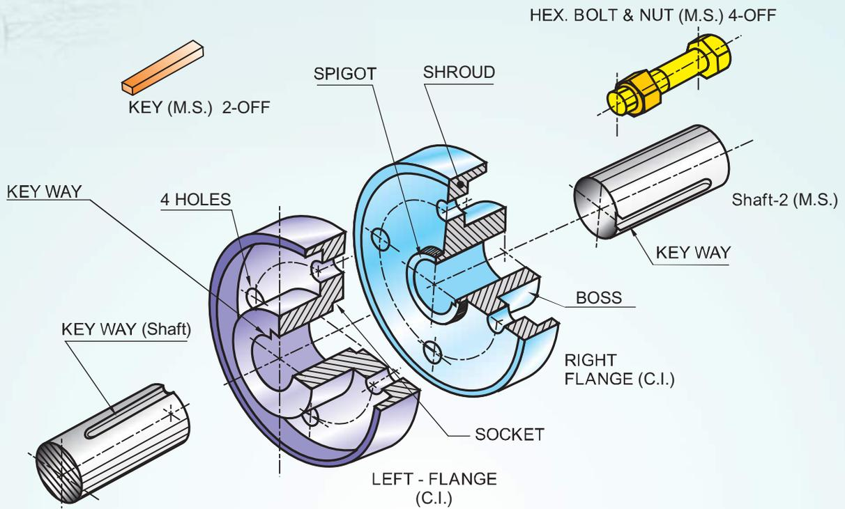
EXPLODED VIEW OF DETAILS OF A PROTECTED FLANGE COUPLING
