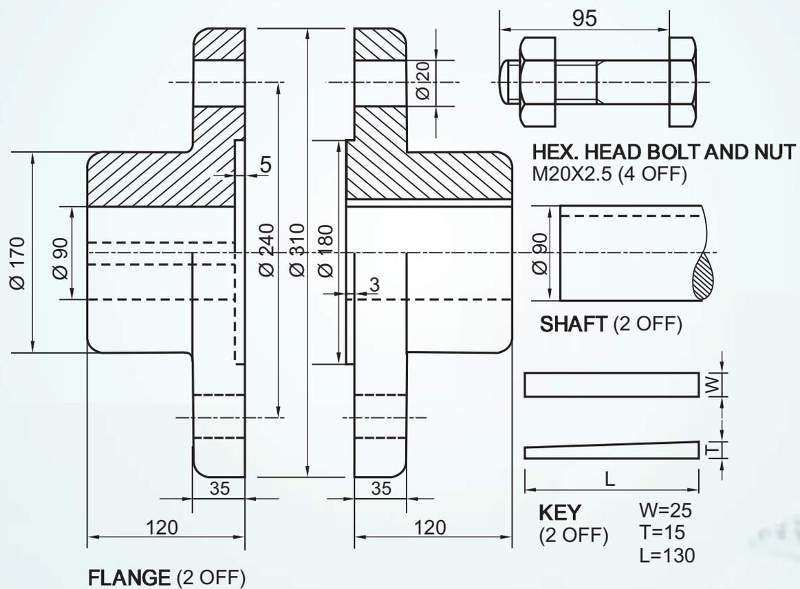
DETAILS OF AN UNPROTECTED FLANGE COUPLING
