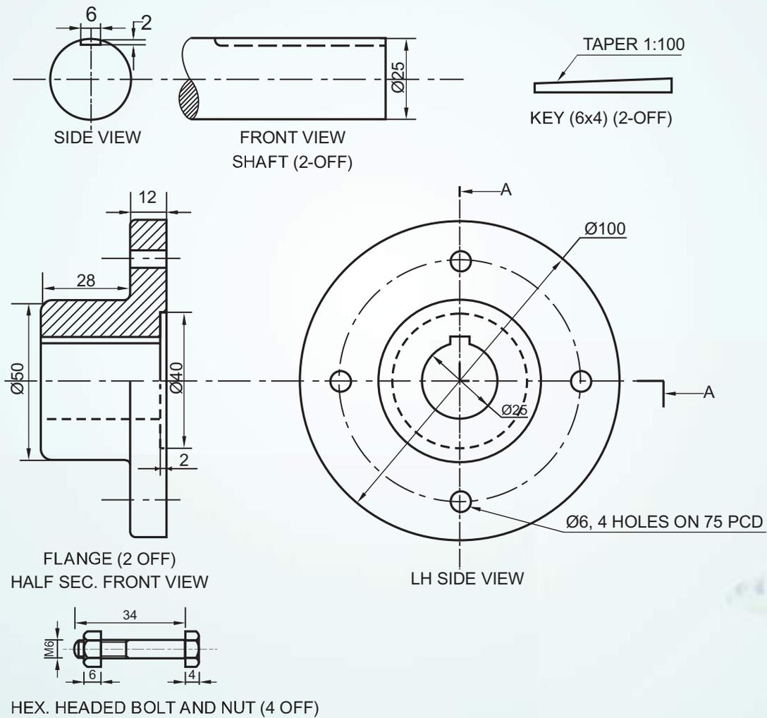
**DETAILS OF AN UNPROTECTED FLANGE COUPLING**
