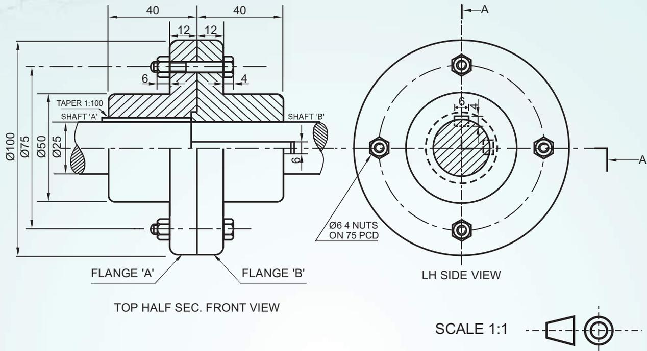
ASSEMBLED VIEW OF AN UNPROTECTED FLANGE COUPLING.
