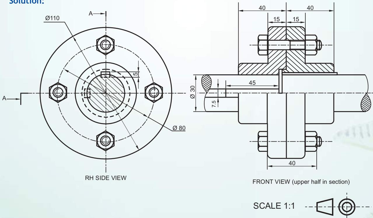
ASSEMBLED VIEWS OF AN UNPROTECTED FLANGE COUPLING
