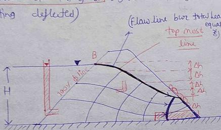
Step ① Focus (F) is the intersect of permeable and impermeable medium.
