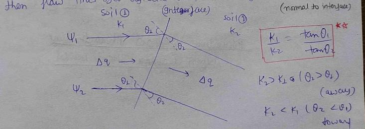
$\theta_1$  and  $\theta_2$  (angle made by flow lines with the normal to interface before and after getting deflected)
