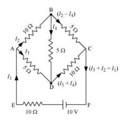
$I_1$  = Current flowing through the outer circuit
