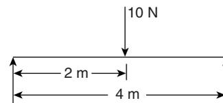
A beam with cross section  $10 \text{ cm}$  width and  $20 \text{ cm}$  depth is loaded as shown in the figure. Maximum shear stress at a section  $1 \text{ m}$  away from end is
