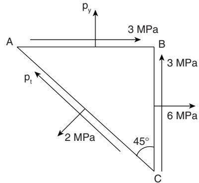
At a point in a stressed body stresses acting are as shown in the figure. Value of  $P_y$  is
