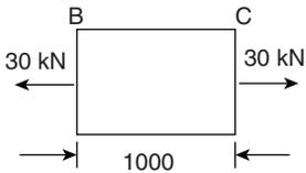
$$\delta l_2 = \frac{p\ell}{AE} = \frac{30 \times 10^3 \times 1000}{1000 \times 1.05 \times 10^5} = -0.2857 \text{ mm (-)}$$
