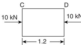
$$\delta l_3 = \frac{p\ell}{A_E} = \frac{10 \times 10^3 \times 1200}{1000 \times 1.05 \times 10^5} = -0.1143 \text{ mm}$$
