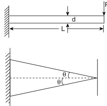
A cantilever beam of varying width and constant depth is loaded as shown in the figure. Maximum bending stress at the fixed end of the beam is
