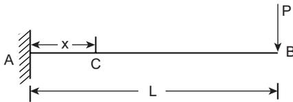
If  $L$  is the length of the beam and  $EI$ , the flexural rigidity, slope at point  $C$  at a distance  $x$  from fixed end is
