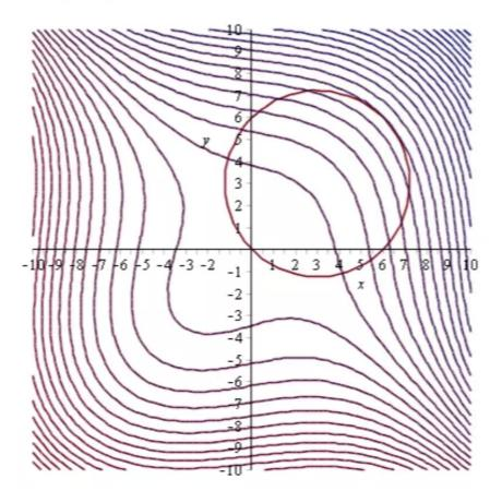
From the contour plot it is clear that, the function has a minimum value at nearly (0.87, 0.87) and maximum value at (5.12, 5.12).
