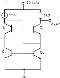
1.21. In figure, both transistors are identical and have a high value of beta. Take the dc base-emitter voltage drop as 0.7 volt and KT/q = 25 mV. The small signal low frequency voltage gain  $(V_o/V_i)$  is equal to \_\_\_\_\_\_
