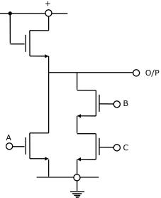
1.28 In figure, the Boolean expression for the output in terms of inputs A, B and C when the clock 'CK' is high, is given by \_\_\_\_\_
