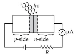
The number of charge carriers increases when light of suitable frequency is made to fall on the  $p$ - $n$  junction, because new electron holes pairs are created by absorbing the photons of suitable frequency. Intensity of light controls the number of charge carriers. Due to this property photodiodes are used to detect optical signals.
