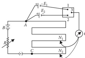
Application of potentiometer for comparing emf's of two cells : The given figure shows an application of the potentiometer to compare the emf of two cells of emf  $E_1$  and  $E_2$ .  $E_1, E_2$  are the emfs of the two cells and 1, 2, 3 form a two way key.
