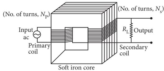
An alternating potential ( $V_p$ ) when applied to the primary coil induced an emf in it.
