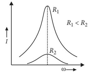
For fine tuning in the receiver set, combination  $L_1 C_1$  and  $R_1$  is better because maximum current flows through the circuit.
